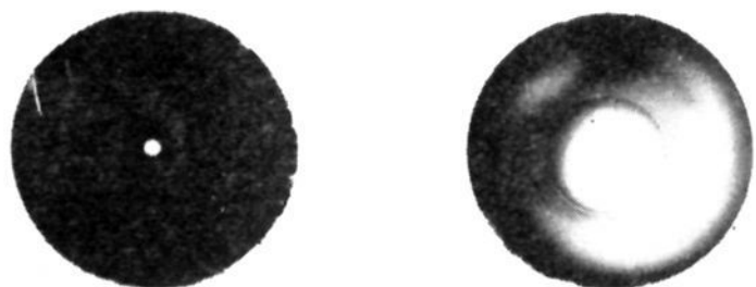
Fig. 3.—End-on photographs of the reaction vessel showing sodium vapor burning in nitrous oxide in absence of carbon monoxide (run 2, to left) and in presence of carbon monoxide (run 4, to right). The photographic conditions were identical.
